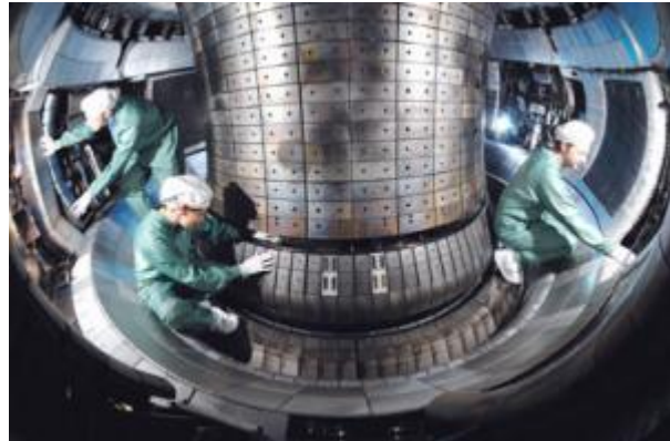
Incorporation of control coils in the plasma vessel of the ASDEX Upgrade fusion device. (Credit: IPP; Volker Rohde)
