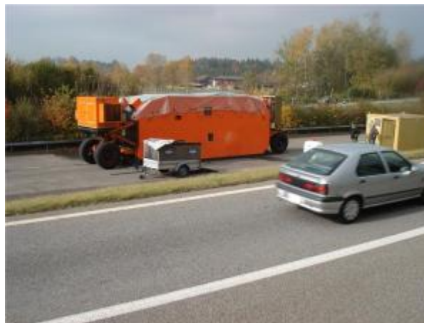
Empa's Traffic Load Simulator during field trials. (Credit: Image courtesy of Empa)
